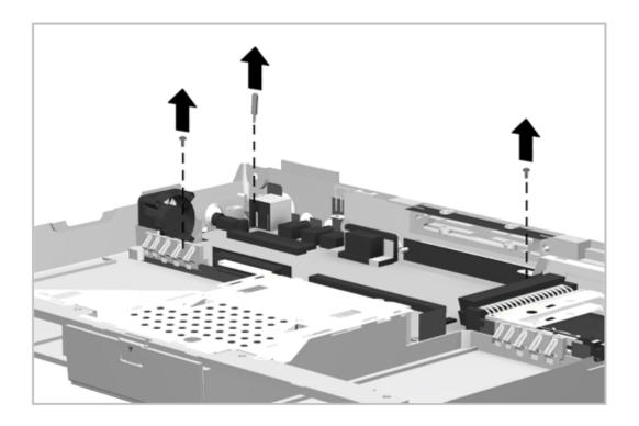
Figure 5-57. Removing the System Board Standoff and Screws
